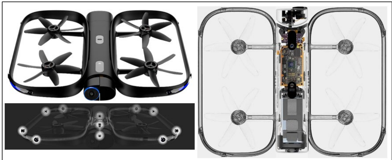
Figure 1: (Left) 13 Cameras Enabling Full 360 ° Vision, Continuous Target Tracking, and Obstacle Avoidance [9, 10] and (Right) NVIDIA Jetson TK CUDA-Core AI Supercomputer With Fully Integrated Autonomous Software Stack [10].
