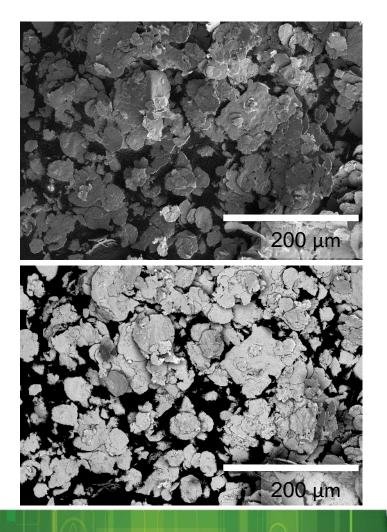
Cryomilled, Degassed, and Sieved (-325 Mesh)
