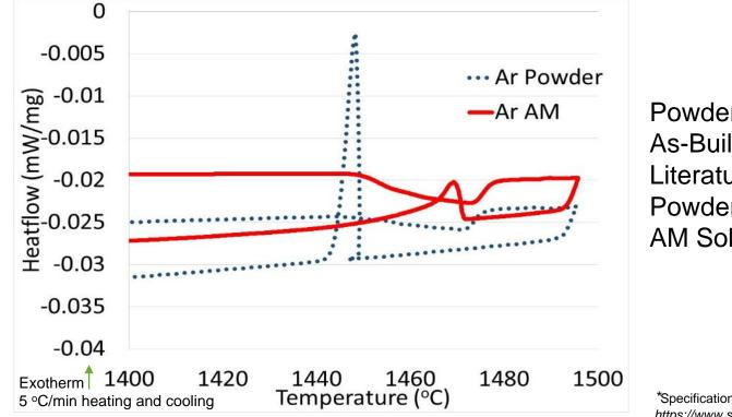
Powder Melting: 1448-1473 °C As-Built Melting: 1450-1478 °C Literature\*: 1404-1440 °C Powder Solidification: 1450 °C AM Solidification: 1472 °C
