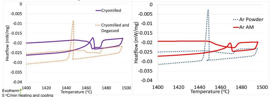
Cryomilled Powder Melting: 1463-1476 °C Degassed Powder Melting: 1458-1473 °C Cryomilled Powder Solidification: 1468 °C Cryomilled and DG Solidification: 1448 °C
