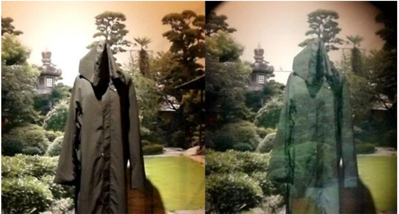
Figure 5-7. Refraction of Light Used to Produce a Cloaking Effect: (Left) a Coat Seen Without a Special Device in Optical Wavelengths and (Right) the Same Coat Seen Through the Half-Mirror Projector Part of the Retroreflective Projection Technology [73].
