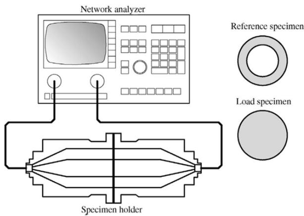
Figure 4-2. ASTM Standard D4935 Is Applied to Measure the SE of Planar Materials (Reproduced From Celozzi et al. [39]).
