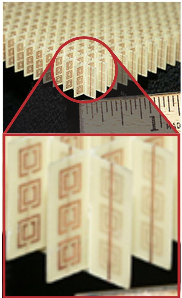
Figure 5-5. Negative-Index Metamaterial Array Configuration Constructed of Copper Split-Ring Resonators and Wires Mounted on Interlocking Sheets of Fiberglass Circuit Board (Source: NASA).
