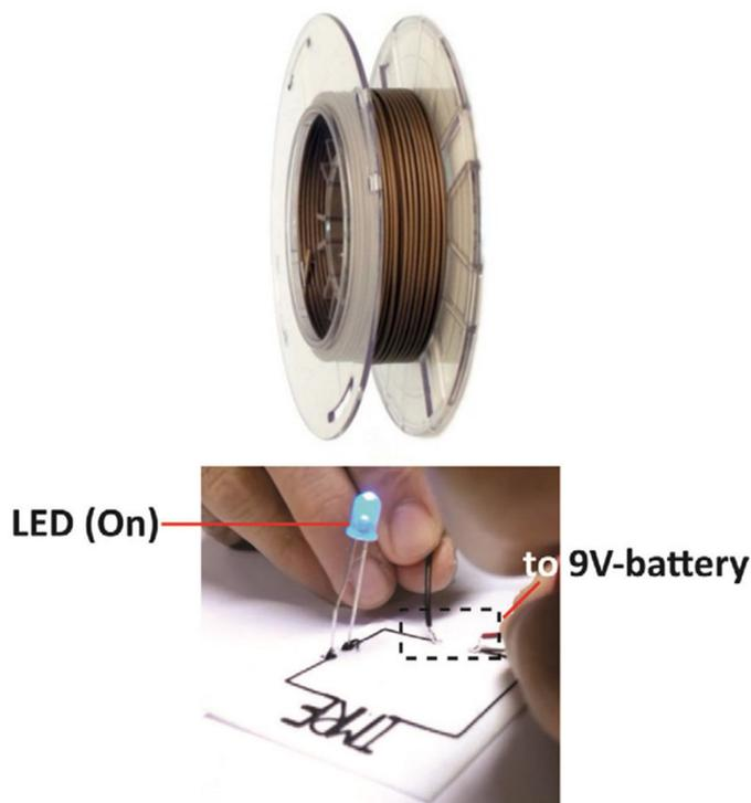
Figure 5-4. Application of Added Conductive Material (Metallic Particles) to Non-Conductive Material (Polymer) for Use as Coatings, Where Copper Is Mixed With Polylactic Acid to Create 3-D-Printed Electronic Circuit Paths [69].
