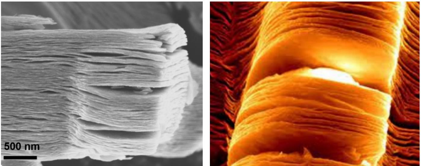
Figure 5-9. Scanning Electron Microscope Images of Layered MXenes (Source: Prussianblue1403).
