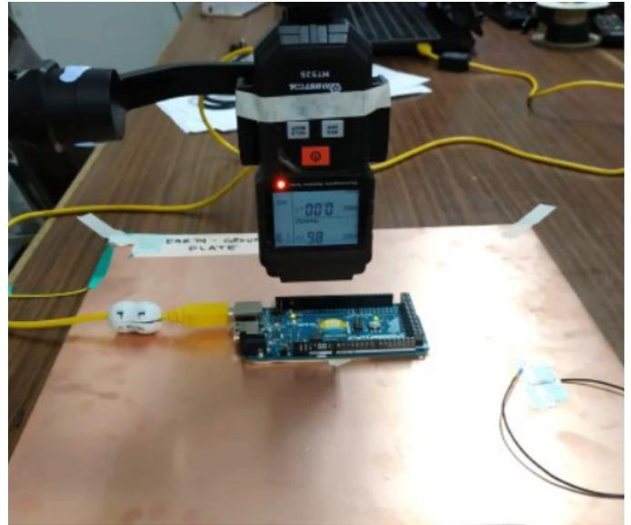
Figure 4-3. Arduino Mega ADK Rev3 Used as the Radiation-Emitting Test Device [64].
