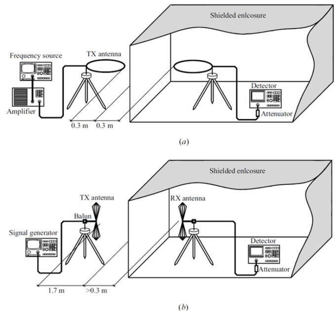
Figure 4-1. IEEE STD-299 Measurement Setup: (a) Low-Frequency Range and (b) Resonant and High-Frequency Range. IEEE STD-299 Is Designed to Measure Shielding of Enclosed Rooms Like a SCIF (Figure Reproduced From Celozzi et al. [39]).
