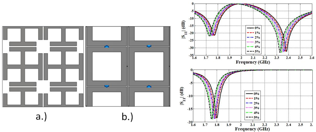
Figure 5-8. Metamaterial Examples Showing How Different Geometries, Configurations, and Circuits Can Produce Different EM Responses: (a) Loaded Cross Dipole Design, (b) Active Rectangular Ring With PIN Diodes (Shown in Blue) and Vertical Bias Lines, (Right Top) Subsequent Sensor Responses for the OFF State, and (Right Bottom) ON State (Source: Doyle Notes).
