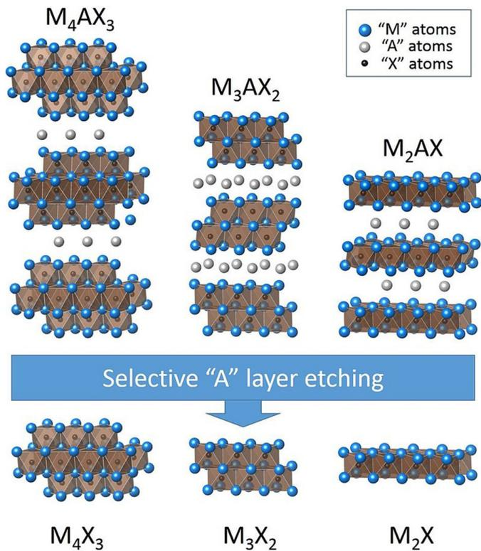
Figure 5-10. MXenes Are Produced by Selective Etching of the "A" Element From the MAX Phase Structure (Source: Prussianblue1403).
