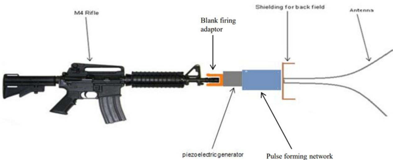
Figure 2-2. Schematic of the M4 Rifle Blank-Firing Attachment With the Piezoelectric Generator Attached [17].
