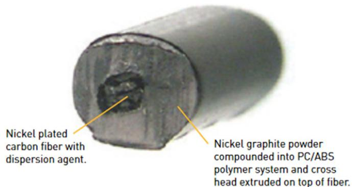
Figure 6-1. Cross Section of Thermoplastic for Injection Molding EM Shielding [83].
