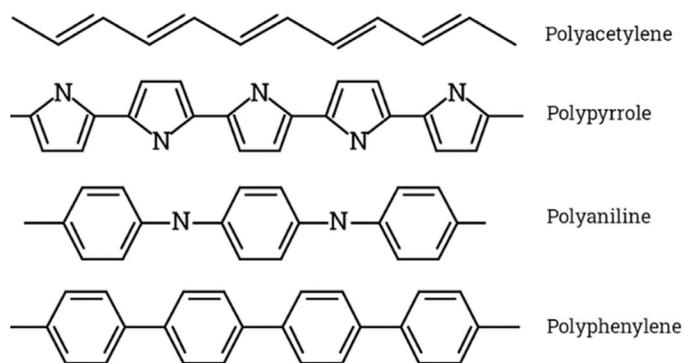
Figure 5-3. Alternating Single and Double Bonds Between Atoms in the Chains of Various Polymers That Can Provide the Bulk Material With Electrical Conductivity (Source: Doyle Notes).
