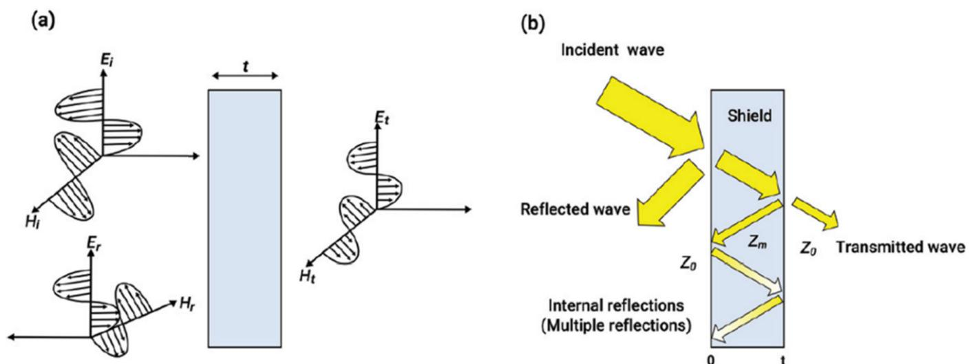
Figure 1-1. (a) A Schematic Illustration of an EM Plane Wave Perpendicular to a Material With a Thickness  $t$  and (b) a Schematic Illustration of the Attenuation of an Incident EM Wave by the Shielding Material (Reproduced from Zhang et al. [1]).
