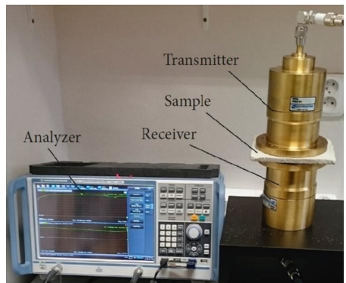
Figure 1-3. Typical Test Setup for Measuring the SE of a Material Sample [5].
