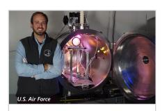
**Multi-Energy Electron Device Creates Space Environment in the Lab**
