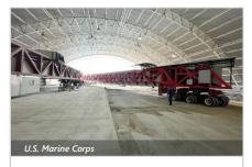
ERDC Begins Testing With World's Largest Heavy Vehicle Simulator
