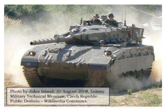
Skirting plates provide effective protection for a small increase in weight. Notice that the skirting plate is relieved where the road wheels can serve the same purpose.
