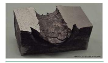
Figure 5-3. Sectioned Perforated Target (Source: Silsby [1]).
