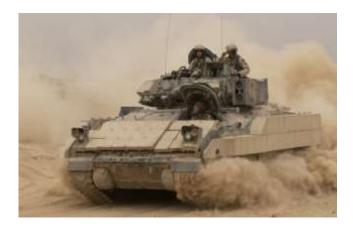
Figure A-10. Bradley IFV with RA Modules (Source: DoD [9]).
