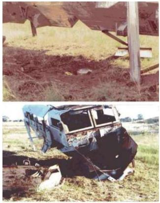
The mine uses 5.1 kg of TNT and penetrates 40 mm of armor at a distance to 800 m and may act sidewise from a distance of 45 m [79].
