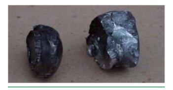
Figure 5-4. Residual Penetrator (left) and Target Plug (right) (Source: Silsby [1]).
