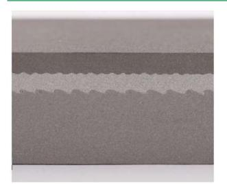
Three plates, explosively bonded. The cut is perpendicular to the collision line. The interlocking "breaking wave" patterns, similar to the familiar Greek stepped-fret motif, are caused by vortices forming and then being crushed together. Explosion welding can bond otherwise incompatible materials. Photo copyright and courtesy of NobelClad Co., Broomfield, CO. Used by permission.
