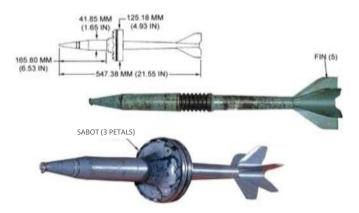
U.S. Navy EOD graphic. Nose has been damaged. Not clear are canted holes in the three sabot petals that impart spin as gun gases are vented up the bore, copper buttons on the substantial steel fins that act as bore riders, and machined leading edges on the fins that create lift to lock the round into a desired roll rate in flight.
