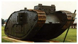
The British Mark II tank of WWI, mounting five Hotchkiss 0.303 light machine guns: two fired from each side and one from the front. No tank since has had such a commodious interior!
