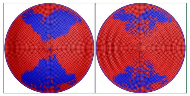
(red indicates delamination - blue indicates tied nodal constraint)
